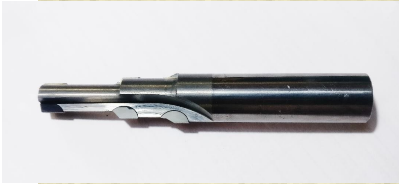
PCD Drill cum combination Reamer.
